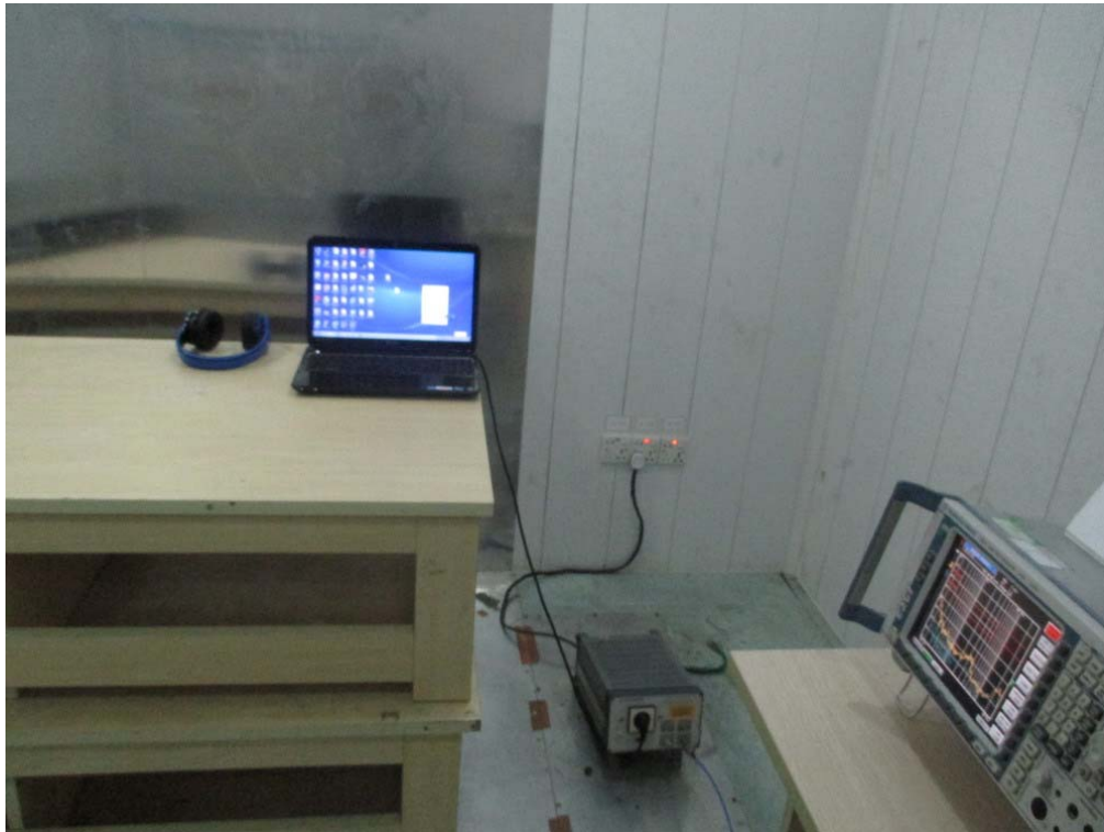
FCC RADIATED EMISSION TEST SETUP
