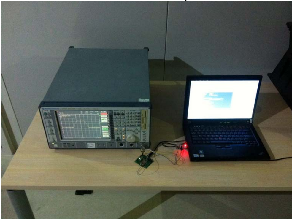
RF Conducted test Setup Photo
