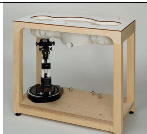
Fig. 8.7 Photo of SAM Twin Phantom
