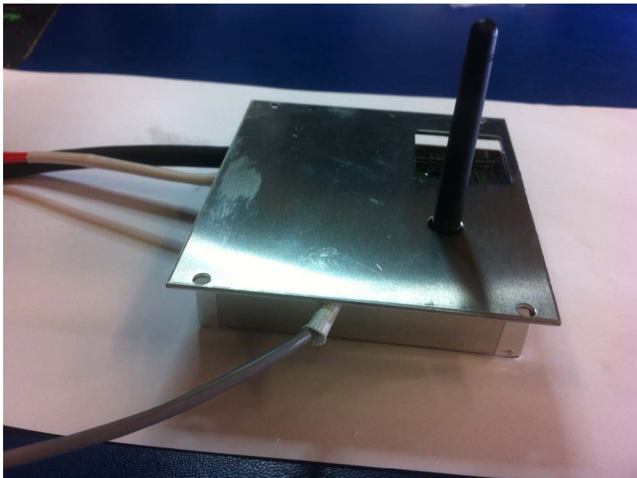
RF Subunit before installation into LED Lighting Assembly
