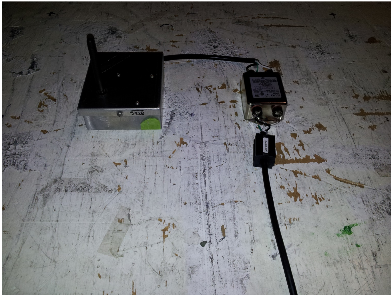
Figure 28:Emissions Test Setup – Intentional / Unintentional Radiated Emissions with Ferrite and AC Filter
