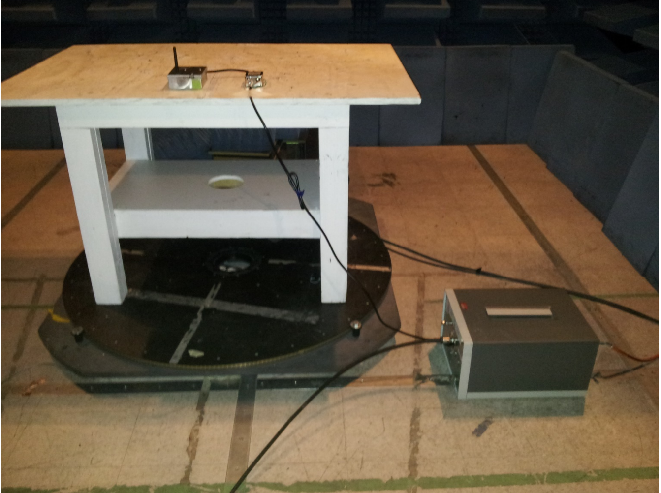
Figure 29:Emissions Test Setup – AC Mains Conducted Emissions
