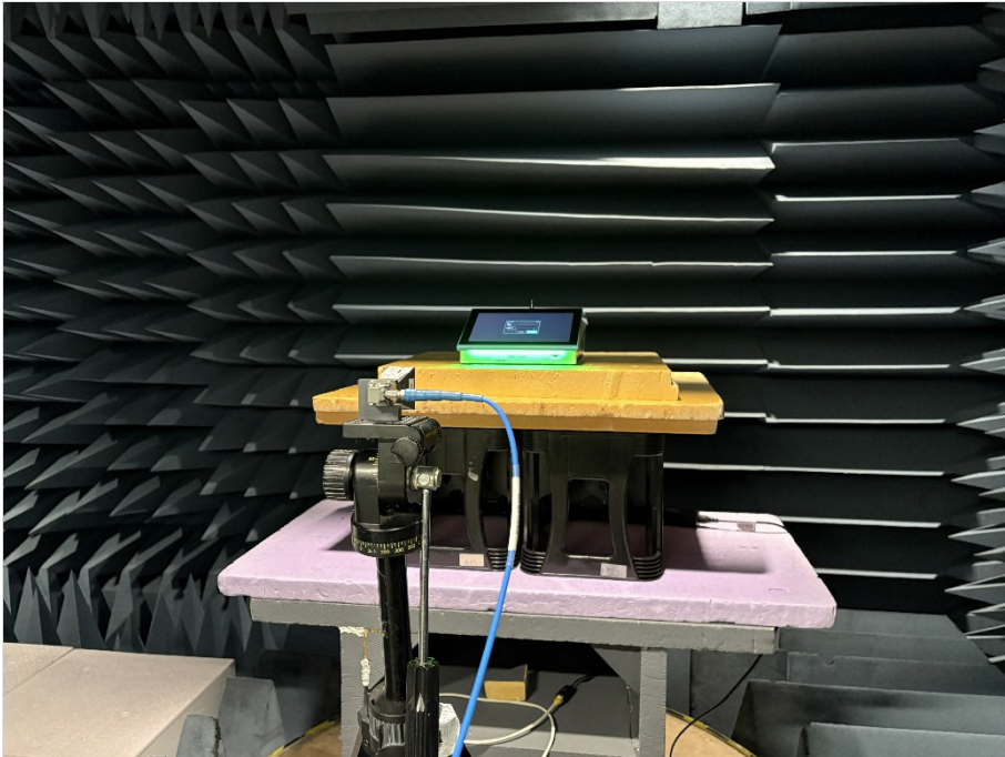
Photograph 3: EUT test setup in the fully anechoic chamber, overview_EUT elevation 0°
