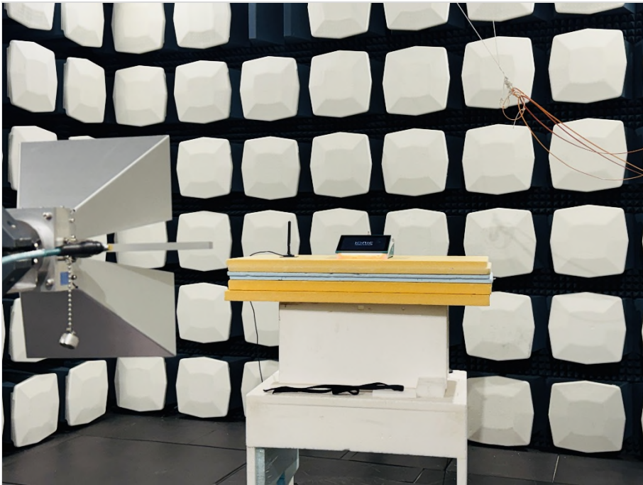
Photograph 1: EUT test setup in the fully anechoic chamber, overview_EUT elevation 0°
