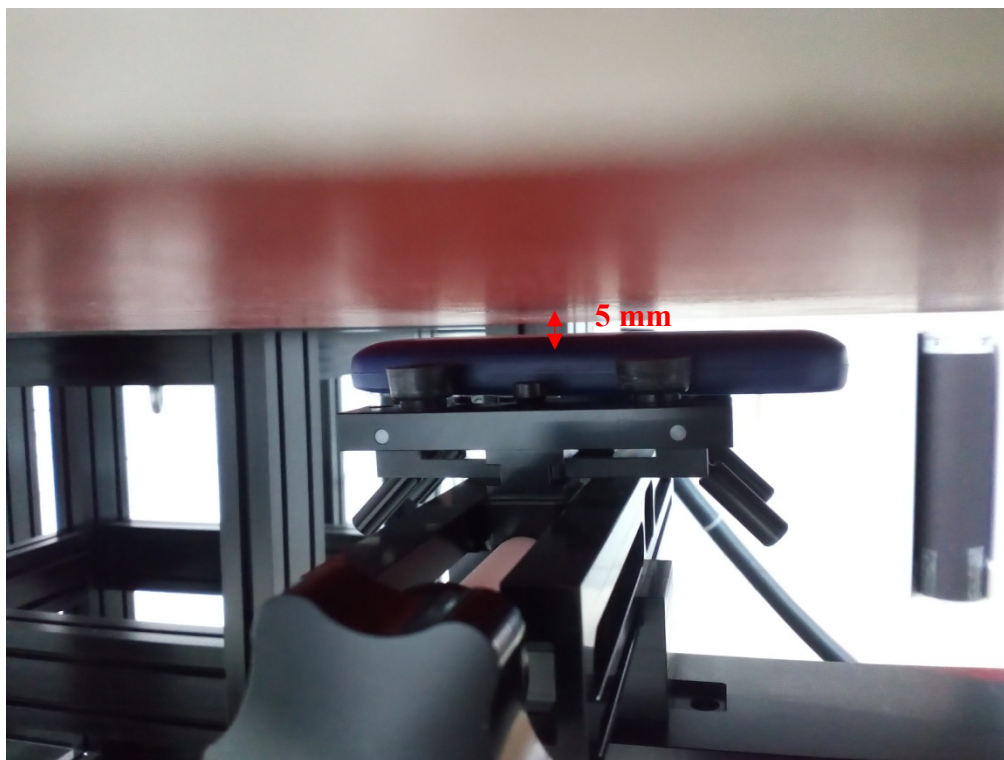
Body (Worn) Back Setup Photo (5mm)
