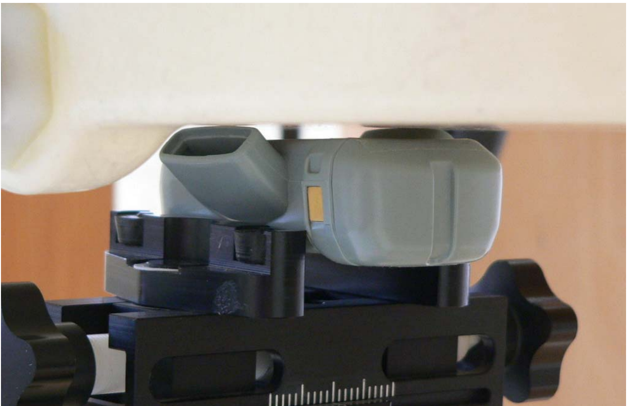
Fig. 11: Back side of OM247 SOLO2 3G 915MHz without the housing, 0 mm distance.
