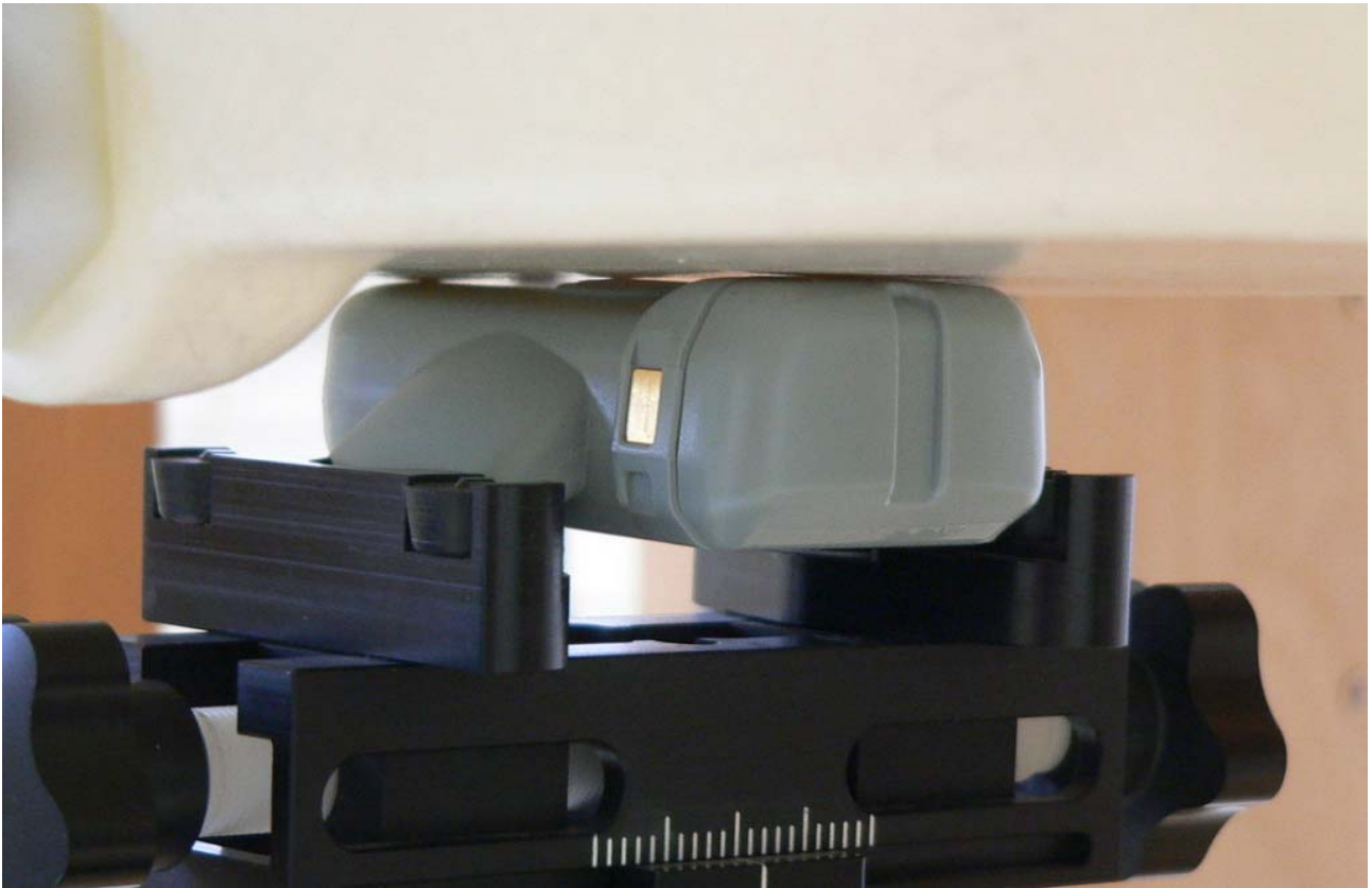
Fig. 10: Front side of OM247 SOLO2 3G 915MHz towards the phantom, 0 mm distance.
