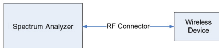
Figure 6-1. Test Instrument & Measurement Setup
