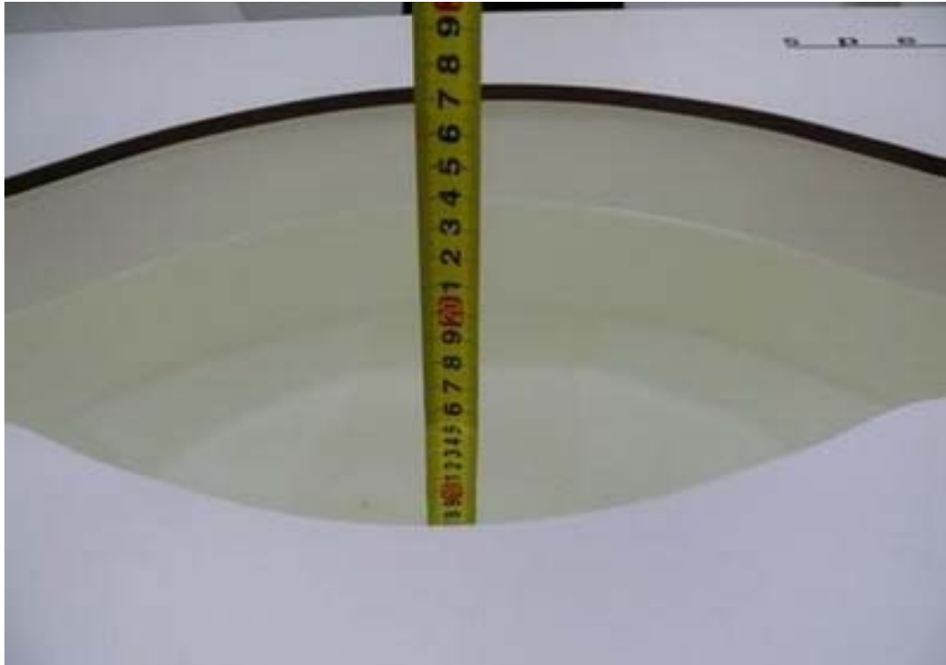
Picture 3: Liquid depth in the flat Phantom
