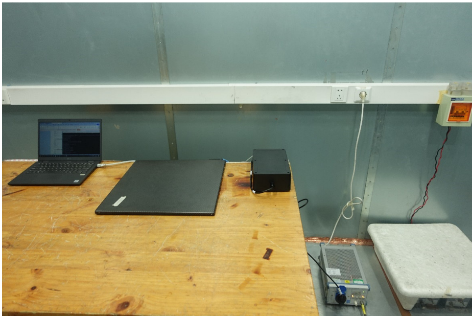
Picture 2 Conducted Emission Test Setup
