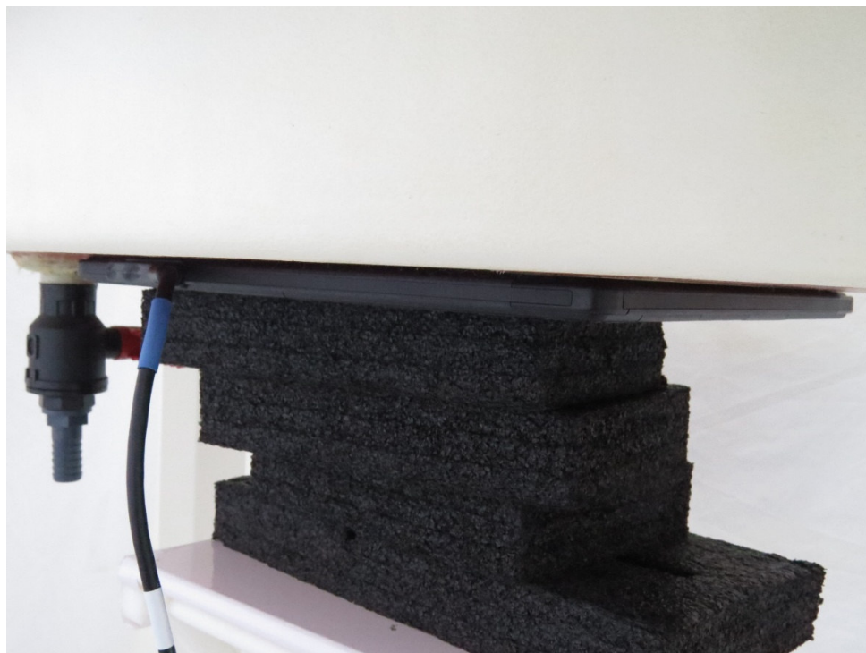
Picture 3: Front Side 3 Zone, the distance from EUT to the bottom of the Phantom is 0mm
