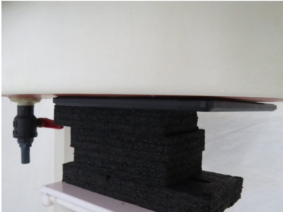
Picture 2: Front Side 2 Zone, the distance from EUT to the bottom of the Phantom is 0mm
