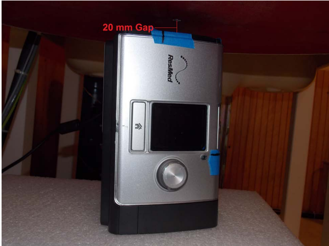
Test Position End 20 mm Gap
