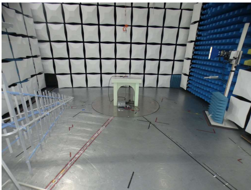
Photo 4: Test setup for radiated measurements below 1GHz
