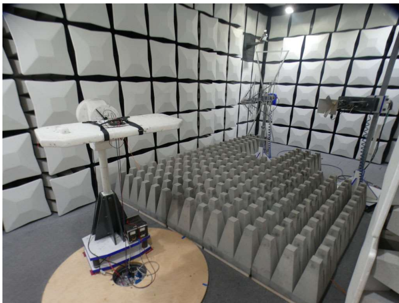
Photo 1: Test setup for radiated measurements above 1GHz
