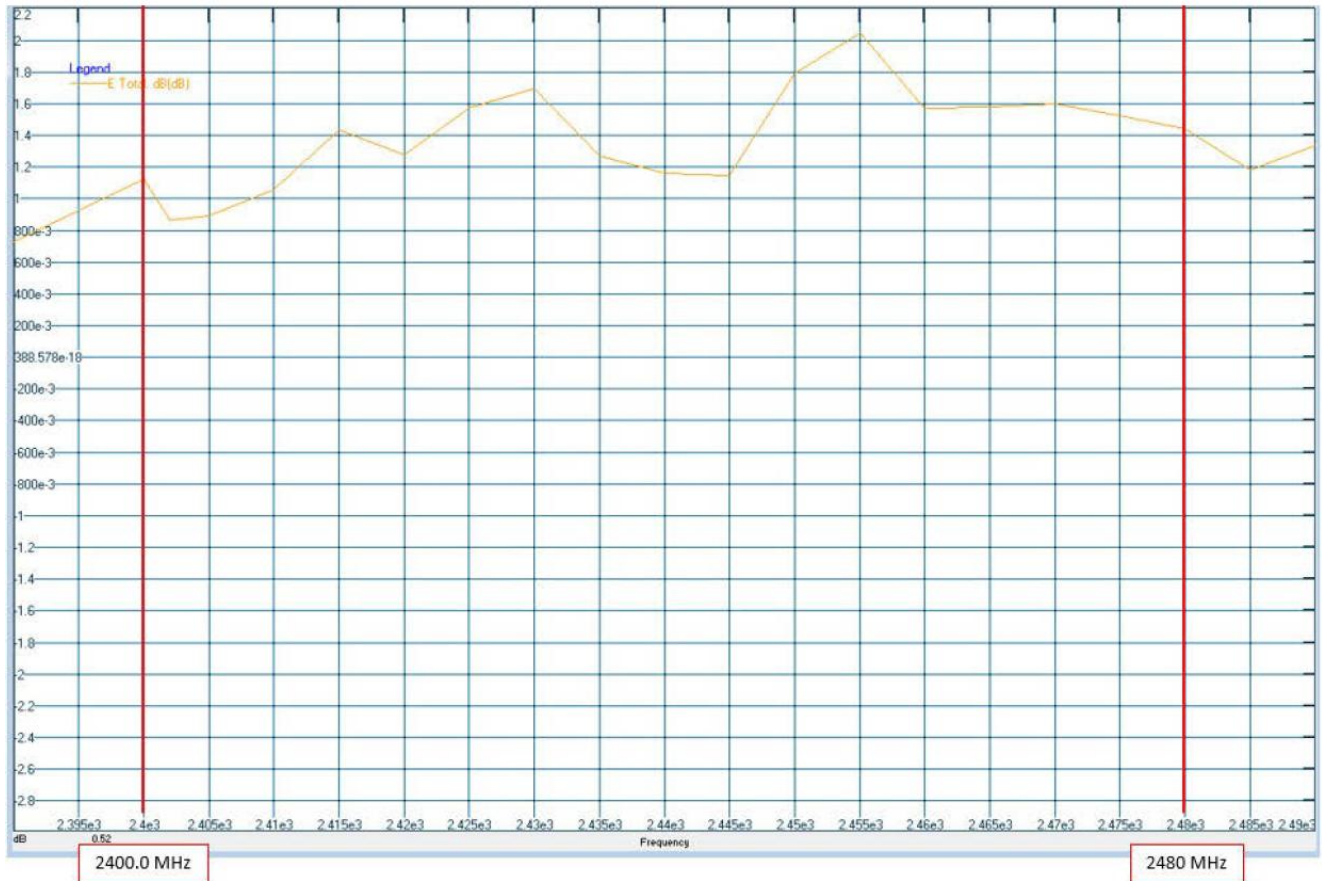
Figure 2. Antenna Gain Related to Frequency
