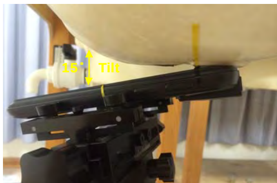
Fig.6 Left Head Section / Ear-Tilt Position(15°)
