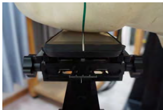
Fig.3 Right Head Section / Cheek-Touch Position
