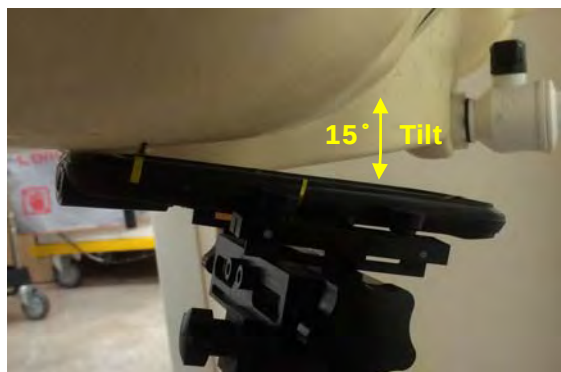
Fig.3 Right Head Section / Cheek-Touch Position
