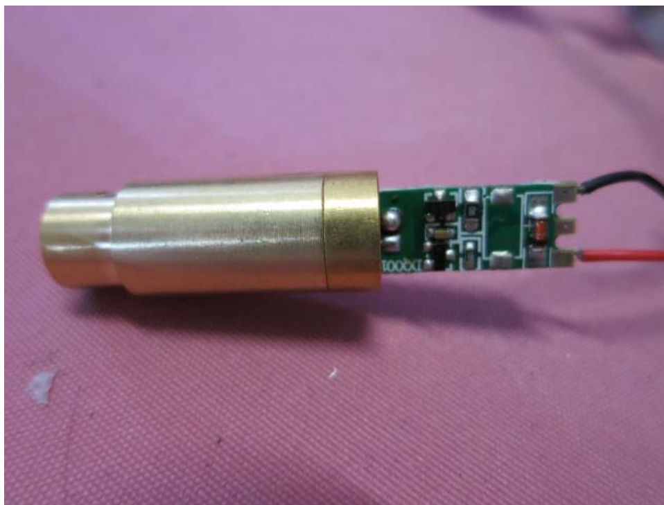
Green Laser Light PCB comp side
