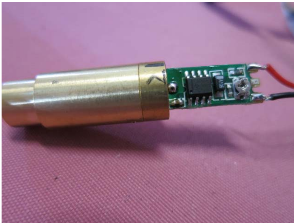
Green Laser Light PCB comp side
