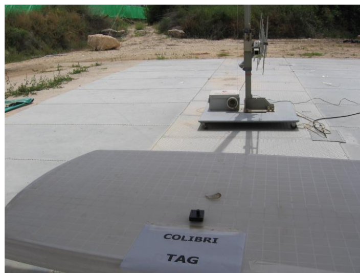
Figure 5. Radiated Emission Test
