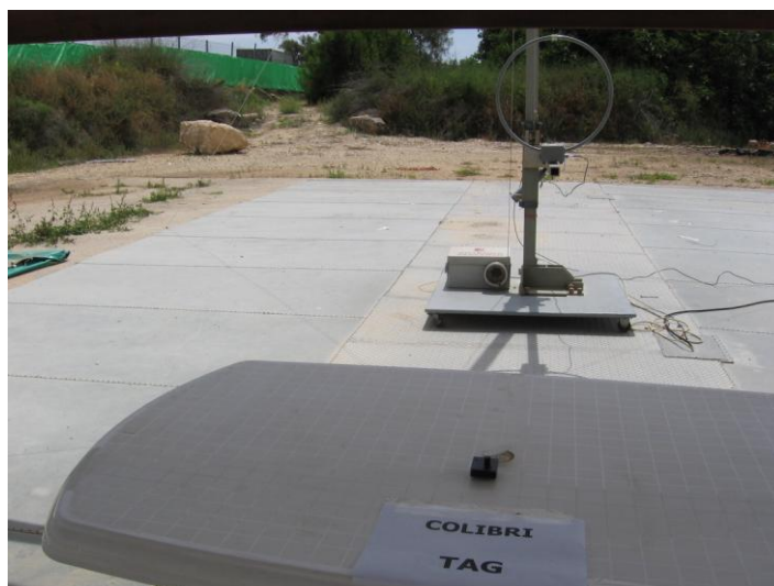
Figure 3. Radiated Emission Test
