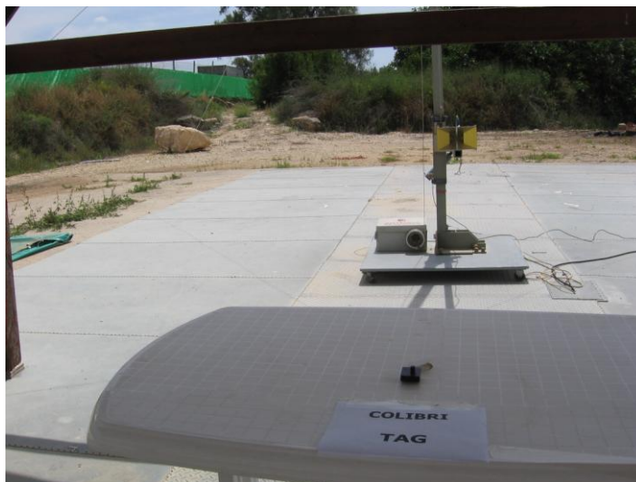
Figure 2. Radiated Emission Test
