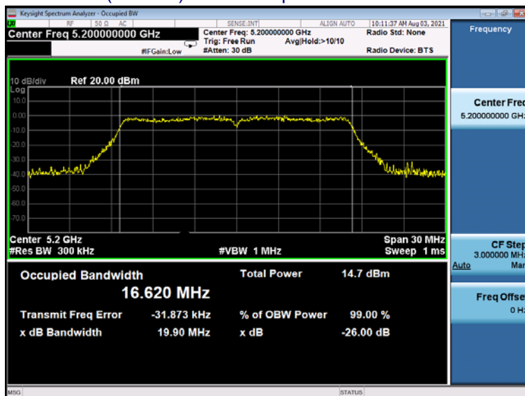
(802.11a) Bandwidth plot on channel 48
