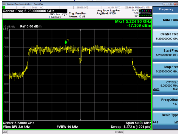
(802.11n40) PSD plot on channel 38
