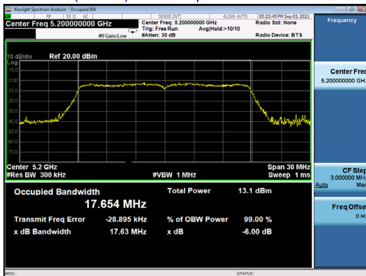
(802.11a) Bandwidth plot on channel 48
