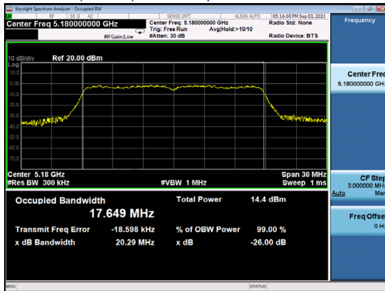
(802.11a) Bandwidth plot on channel 40
