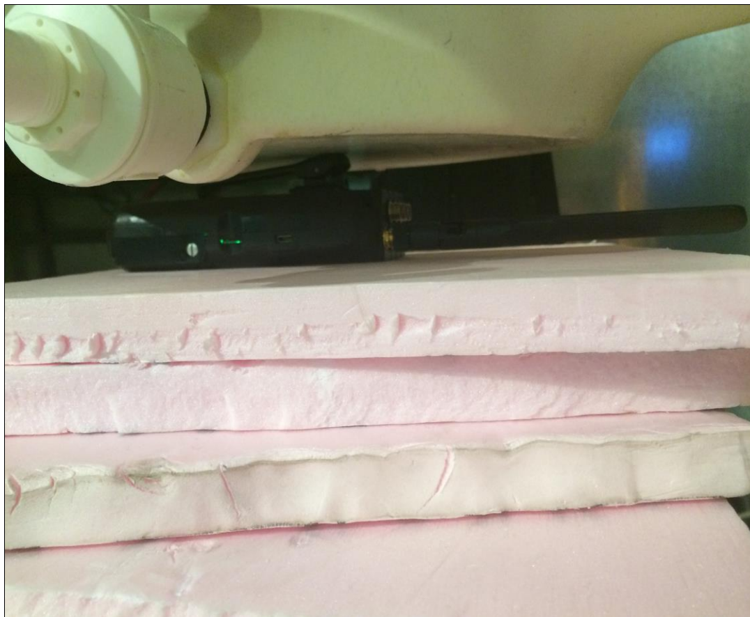
Photograph 2. Back Side of the EUT Against Phantom
