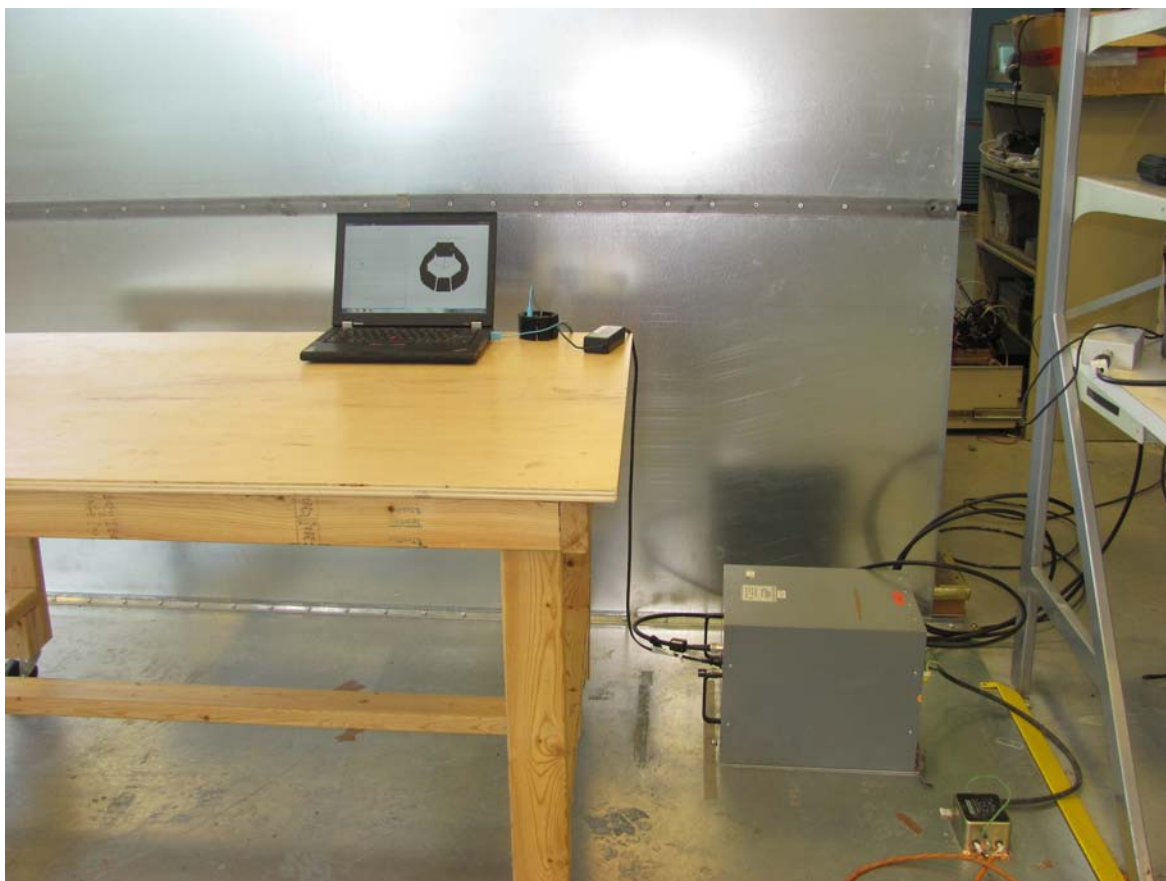
Illustration 7: Power line conducted emission setup – photo 1
