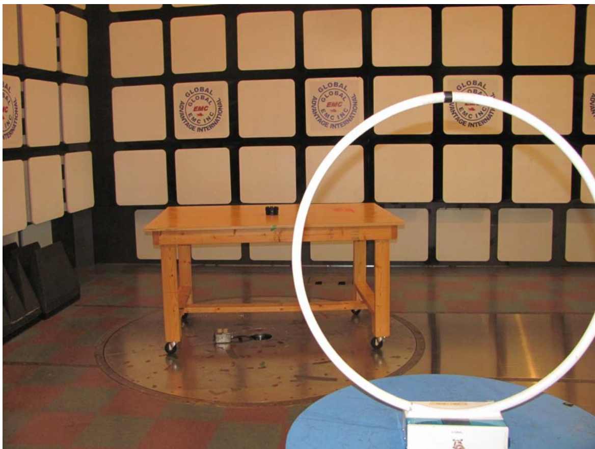
Illustration 3: Radiated emission setup – photo 1
