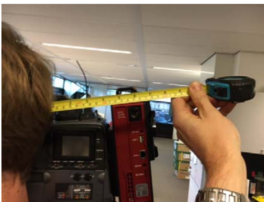
Figure 2: Minimum distance between the head and the unit aerial must be bigger than 2.5 cm using it on the back of a camera
