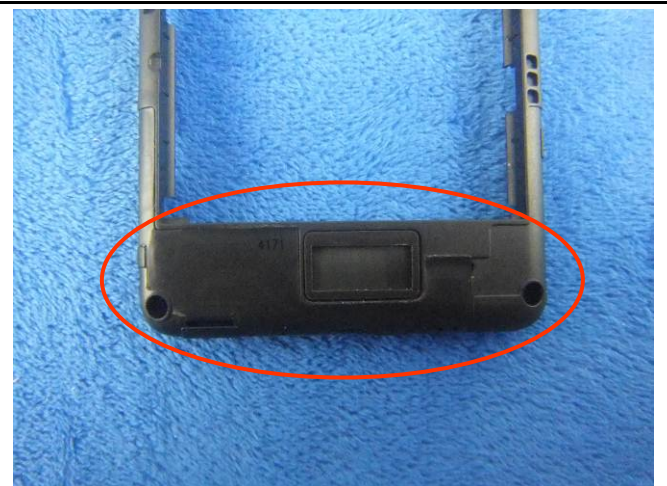
GSM/PCS/UMTS-FDD Antenna View
