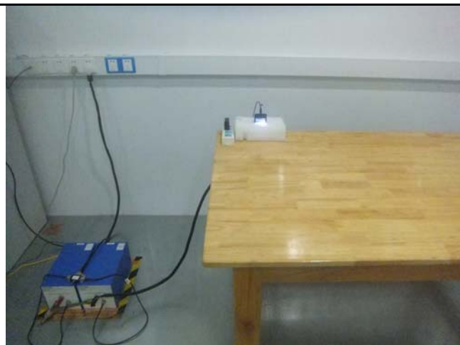
Conducted Emissions Test Setup Front View
