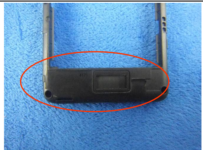
GSM/PCS/UMTS-FDD Antenna View
