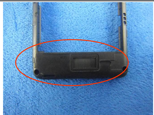
GSM/PCS/UMTS-FDD Antenna View
