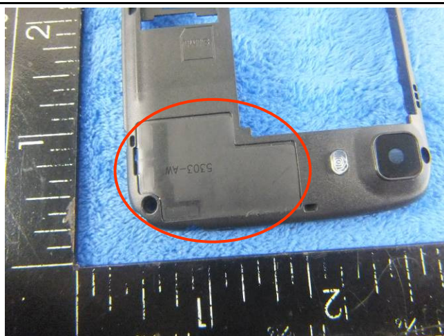
WIFI/BT/BLE/GPS - Antenna View
