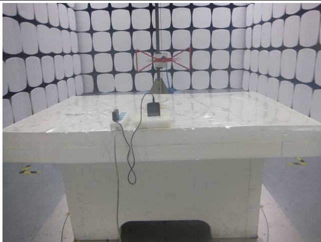
Conducted Emissions Test Setup Front View
