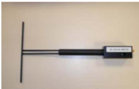
Figure 1 – Satimo COMOSAR Validation Dipole
