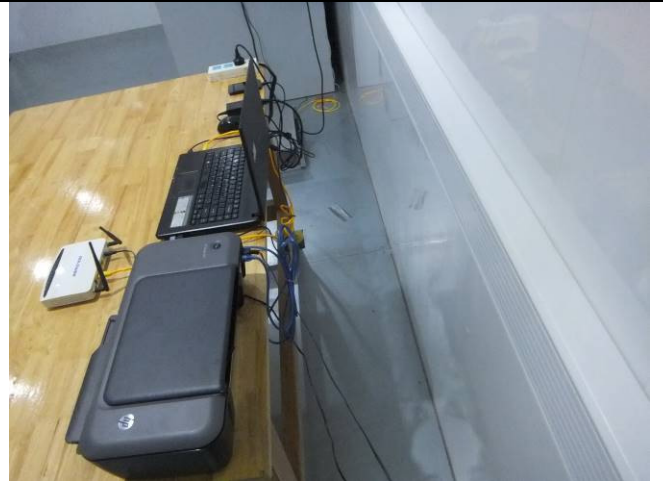
Conducted Emissions Test Setup – Side View
