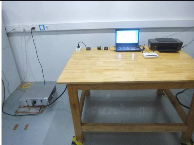
Conducted Emissions Test Setup – Front View
