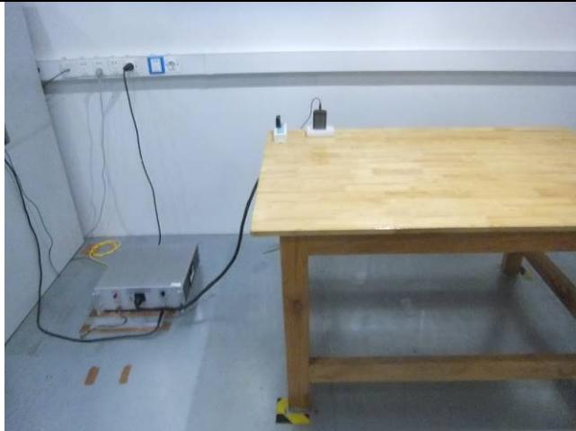
Conducted Emissions Test Setup Front View
