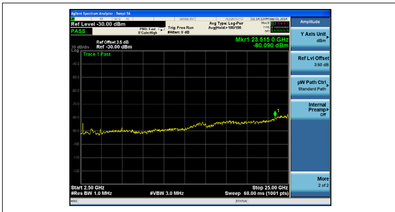
Plot 5.3.4.2.10. Conducted Spurious Emissions for LB Diversity, 2326.256040 MHz, 2.5 GHz – 25 GHz
