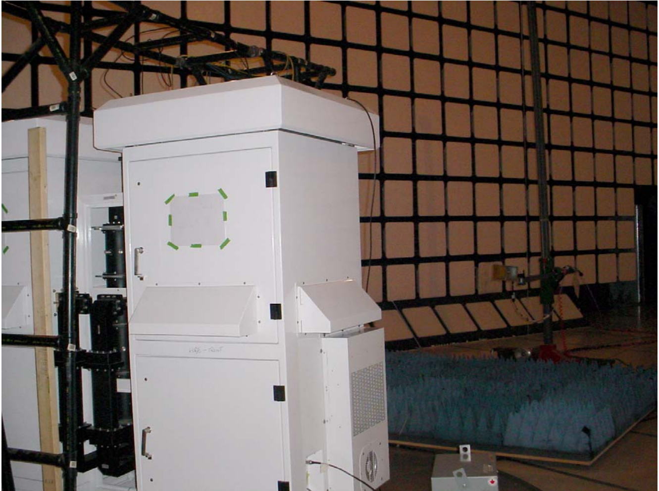
Transmitter Radiated Emission Test at 3m
