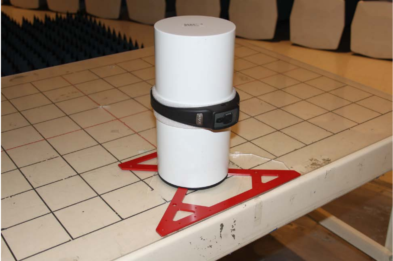
Radiated Emissions Test Setup
