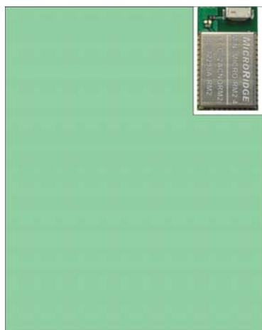
Module placed along top edge of PCB.
