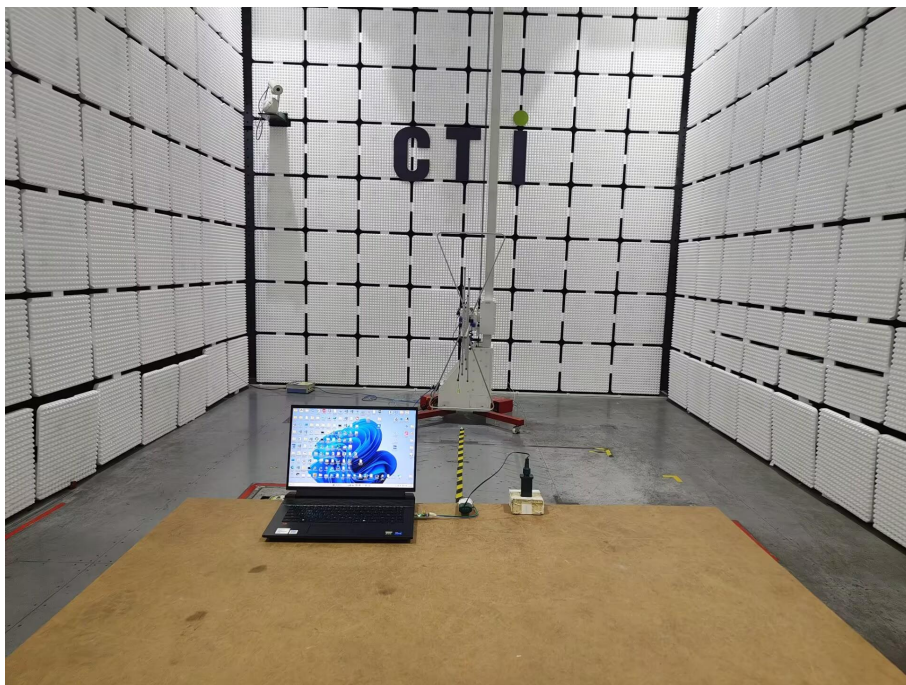
Radiated spurious emission Test Setup-1(Below 1GHz)
