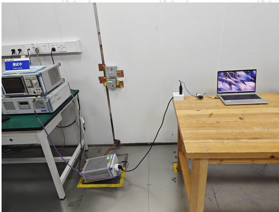
Conducted Emissions Test Setup
