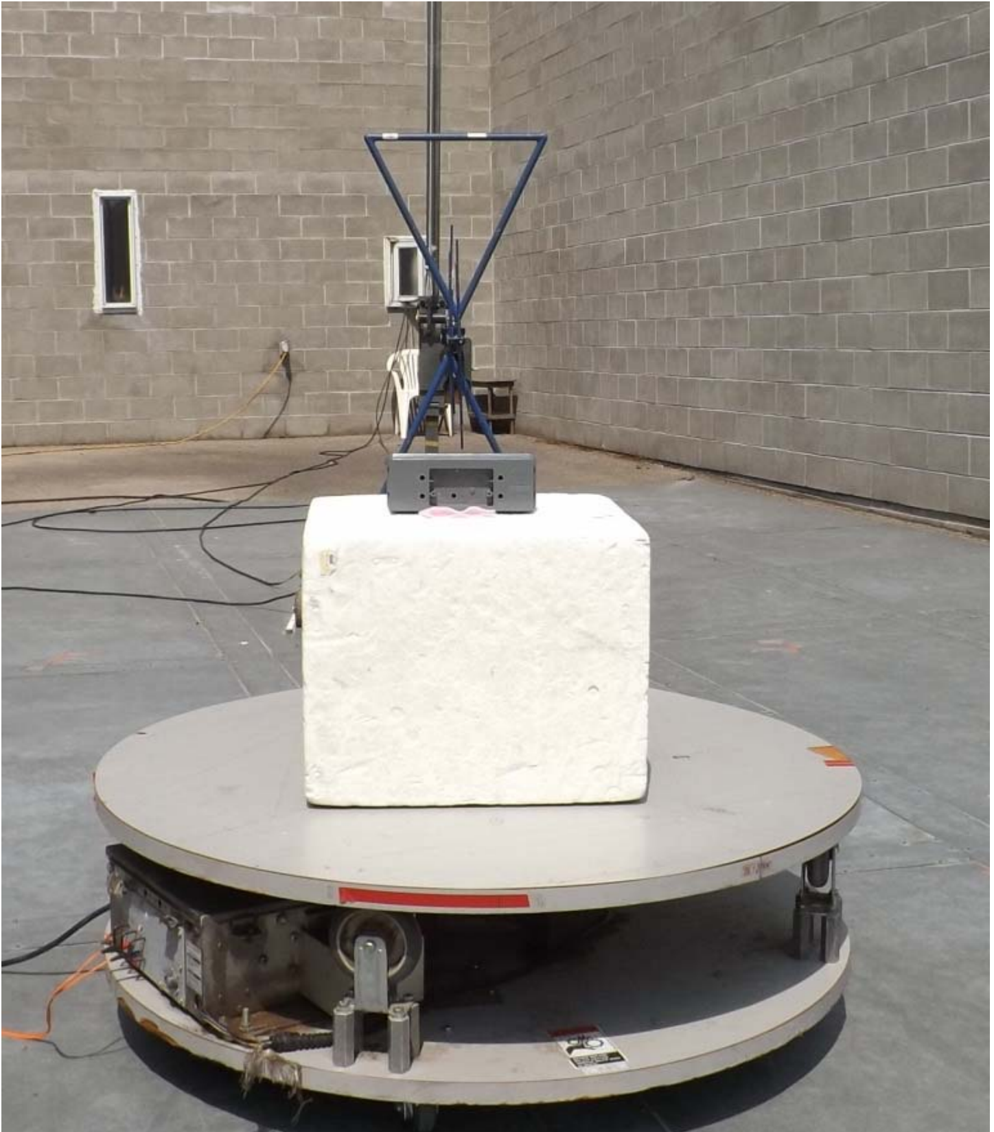
Figure E23.3 – Setup, Radiated Measurements, 30 - 1000MHz
