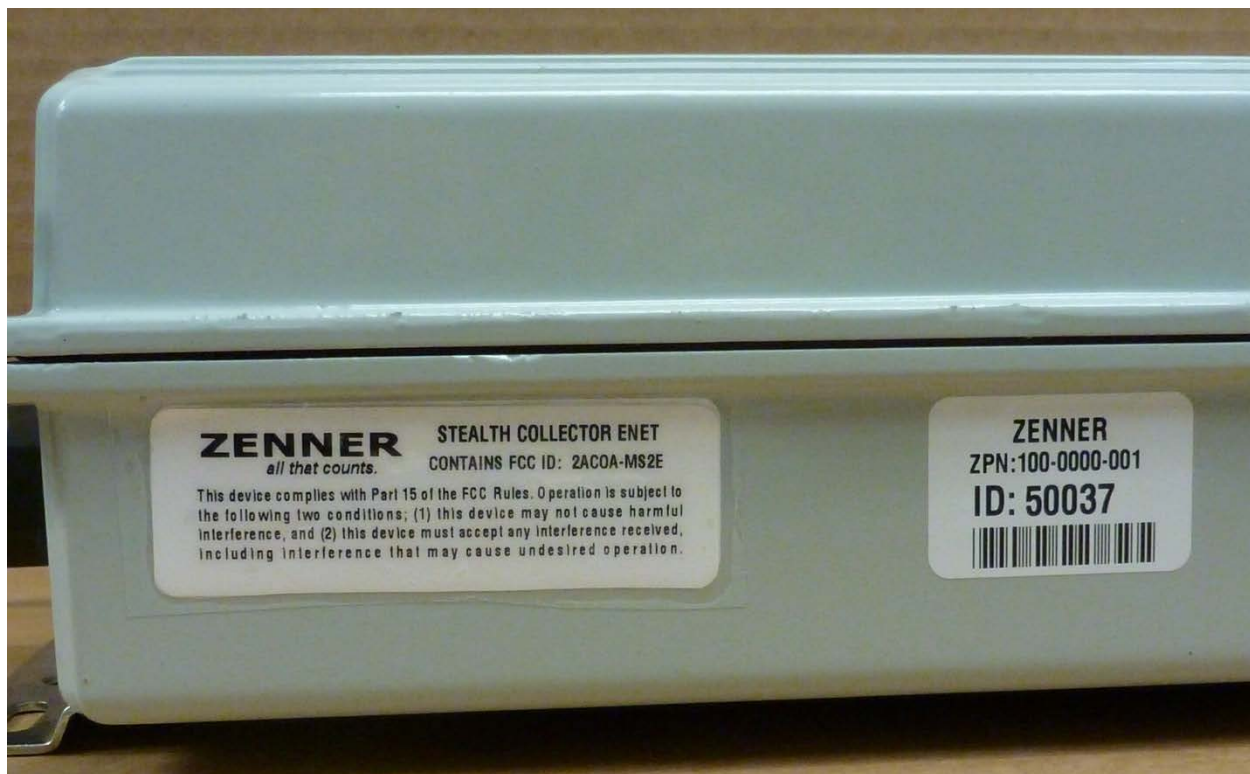
Typical label placement on host for 2ACOA-MS2E
