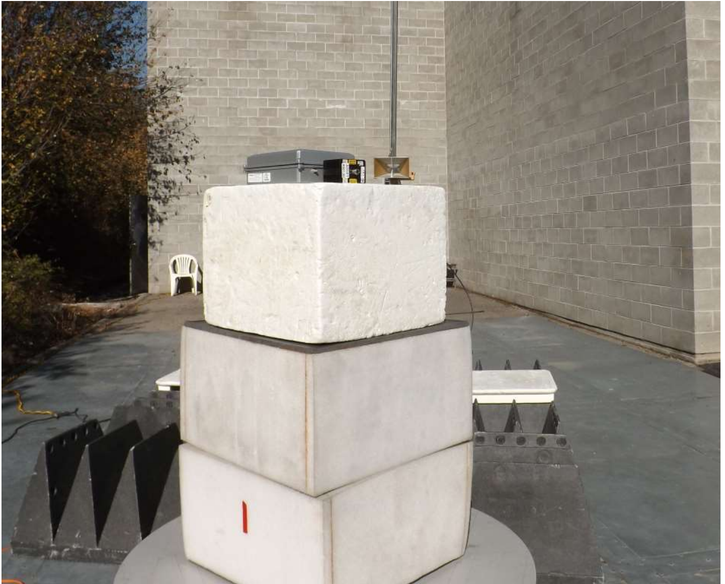
Figure E18.3 – Setup, Radiated Tx 1 - 10GHz
