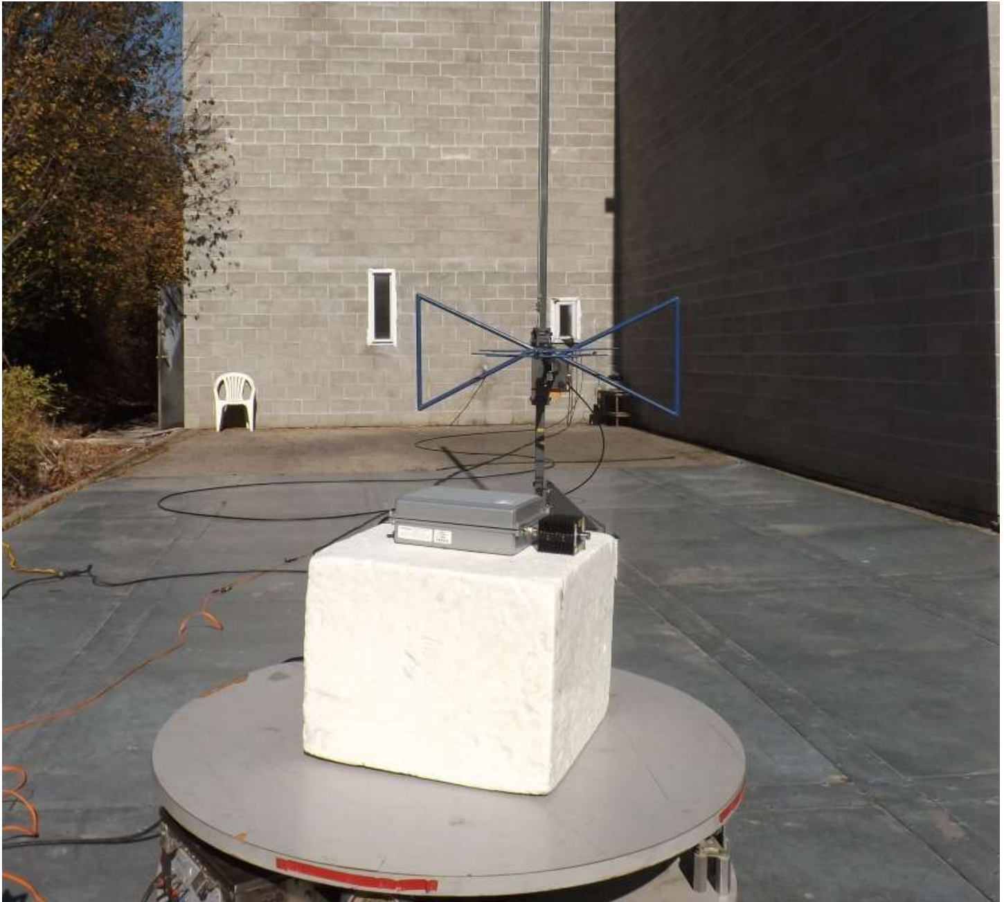
Figure E18.2 – Setup, Radiated Tx 30 - 1000MHz
