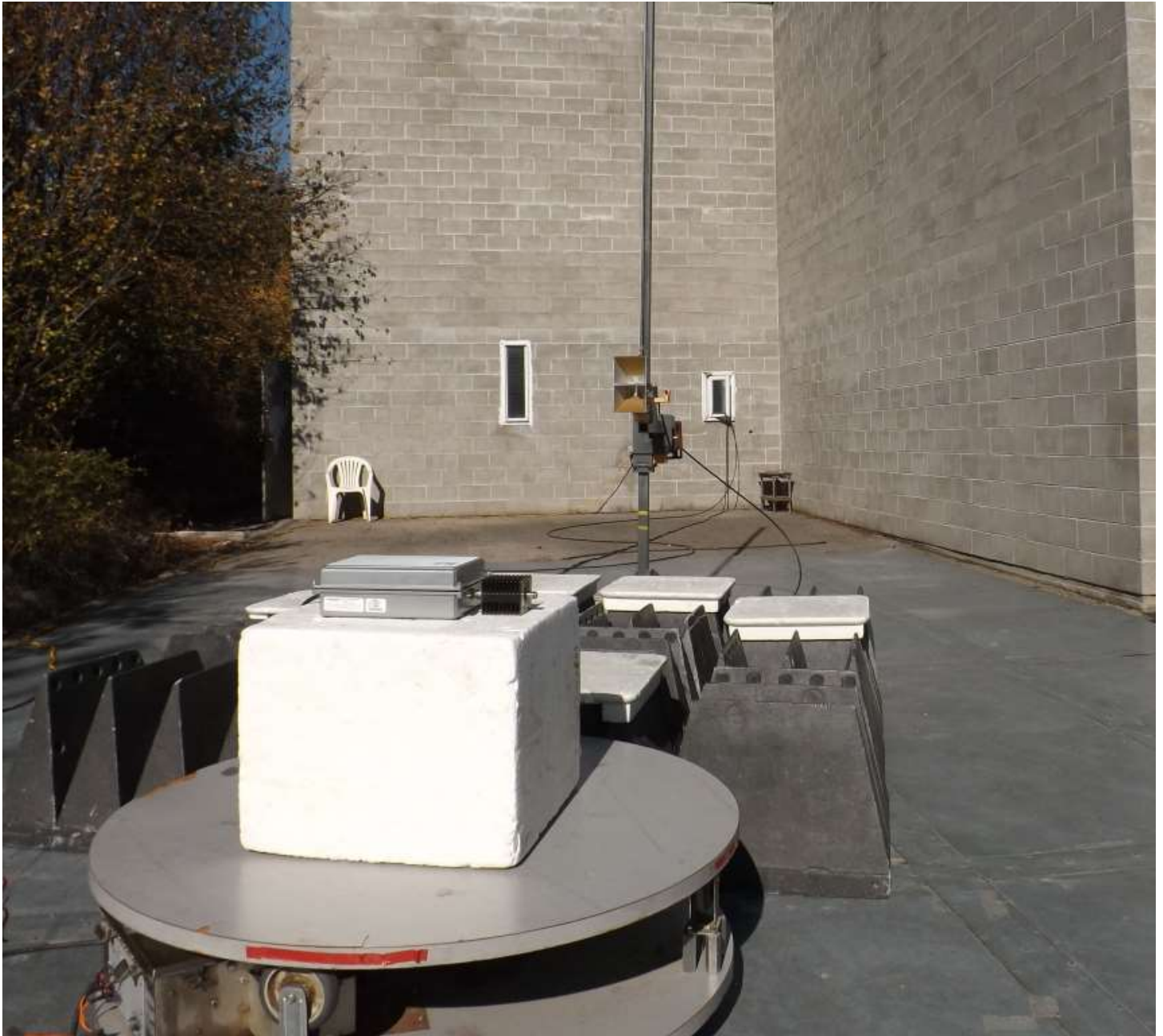
Figure E18.4 – Setup, Radiated Rx 1 - 10GHz
