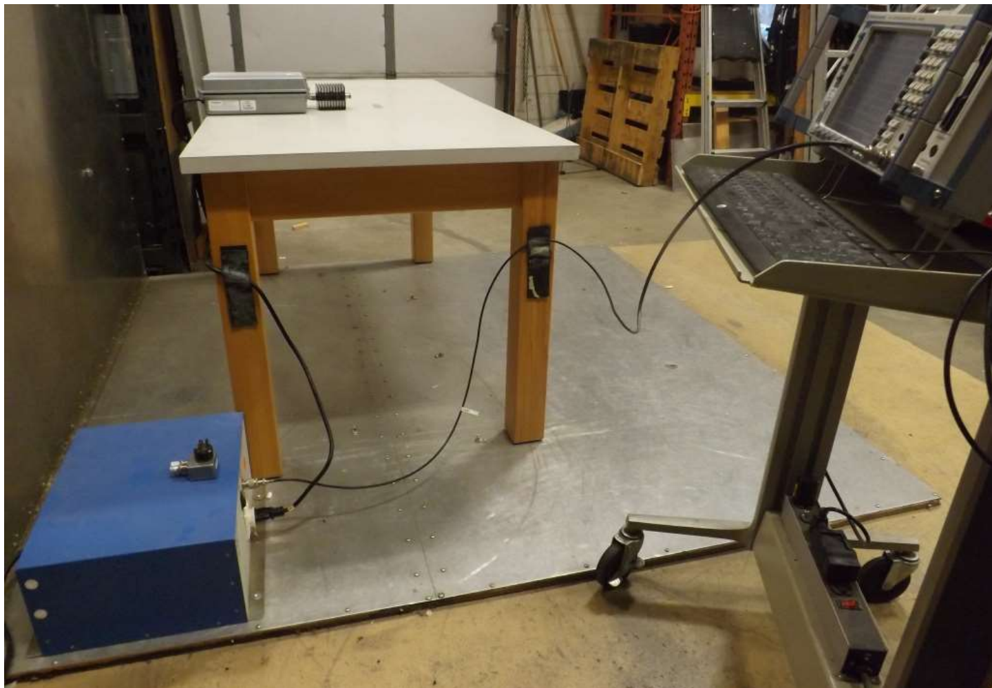
Figure E18.5 – Setup, Line Conducted Emissions
