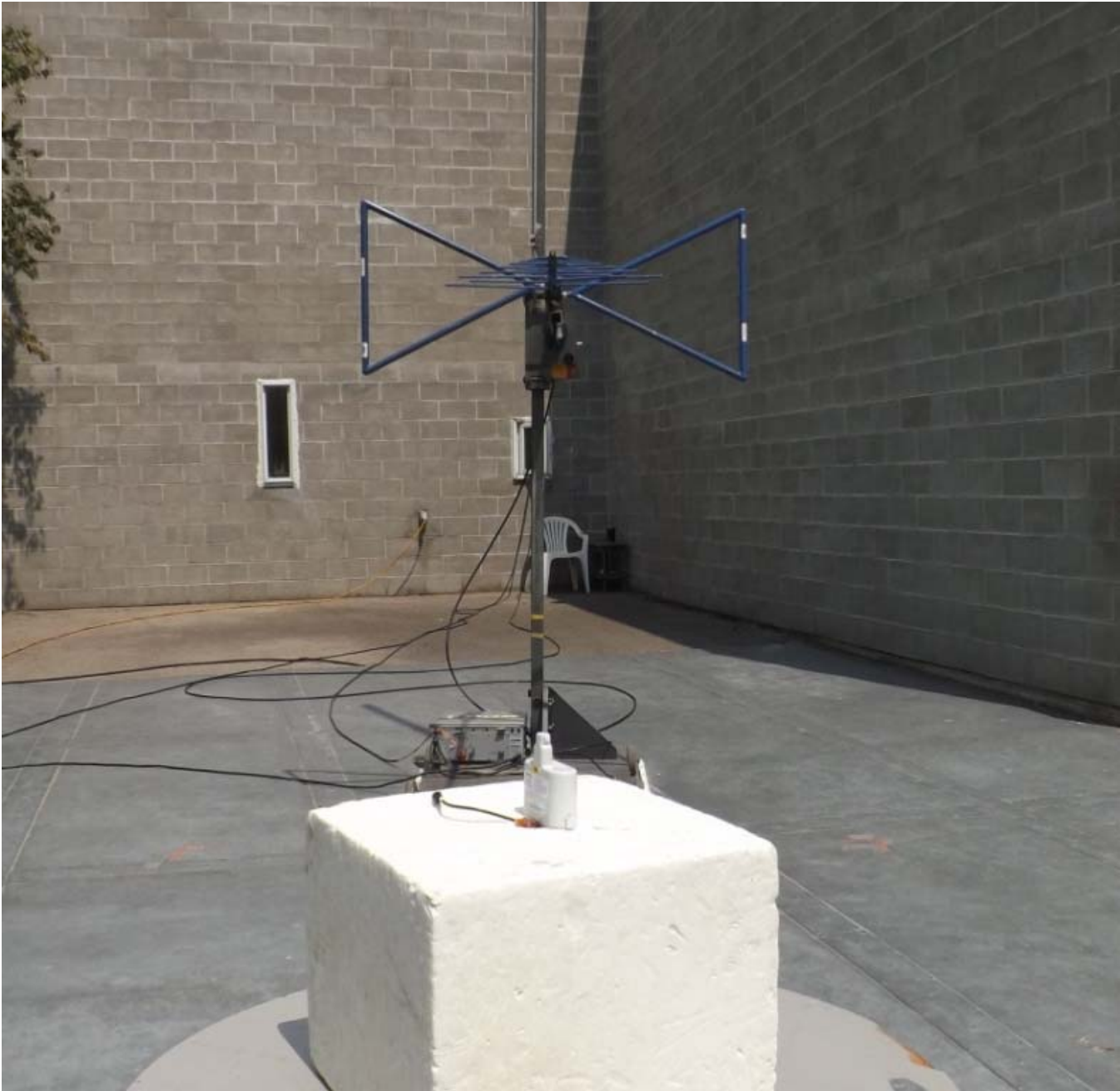
Figure E23.4 – Setup, Radiated Emissions, 30-1000MHz, Horizontal Polarization
