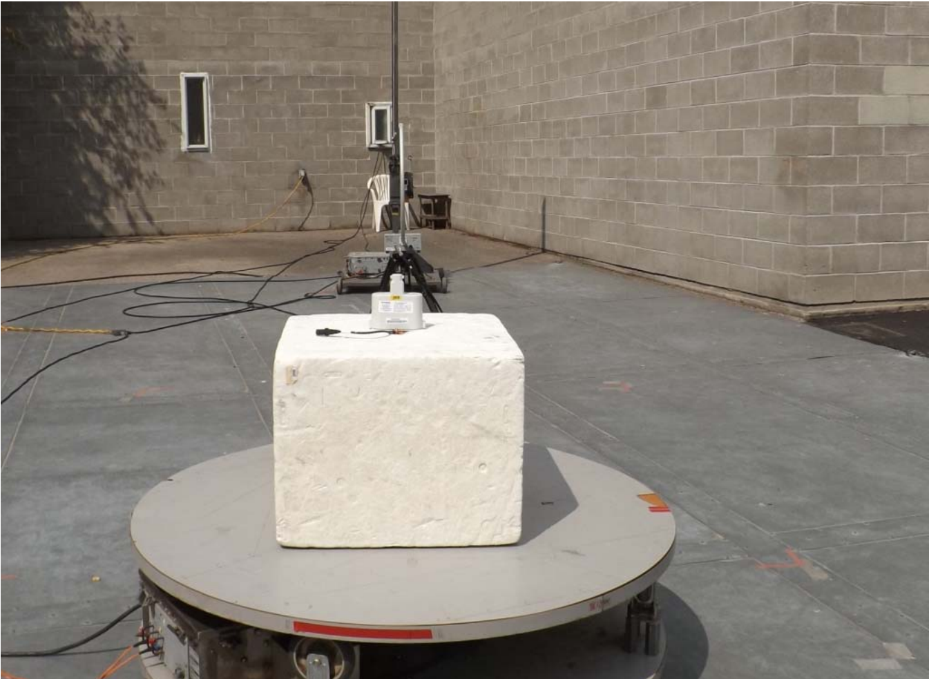
Figure E23.3 – Setup, Radiated Emissions, 9kHz-30MHz, Side Polarization
