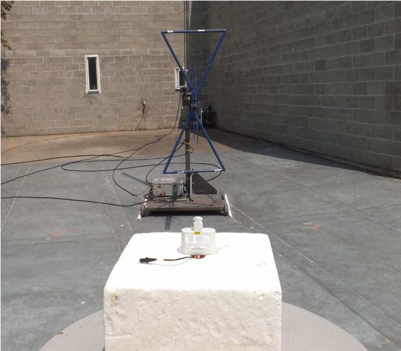
Figure E23.5 – Setup, Radiated Emissions, 30-1000MHz, Vertical Polarization
