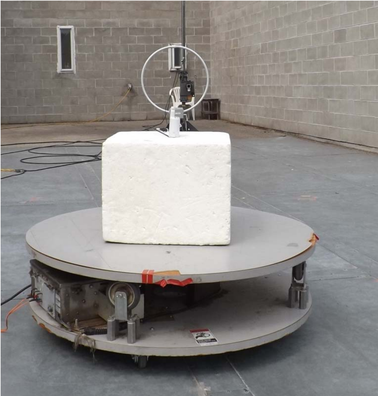
Figure E23.2 – Setup, Radiated Emissions, 9kHz-30MHz, Front Polarization
