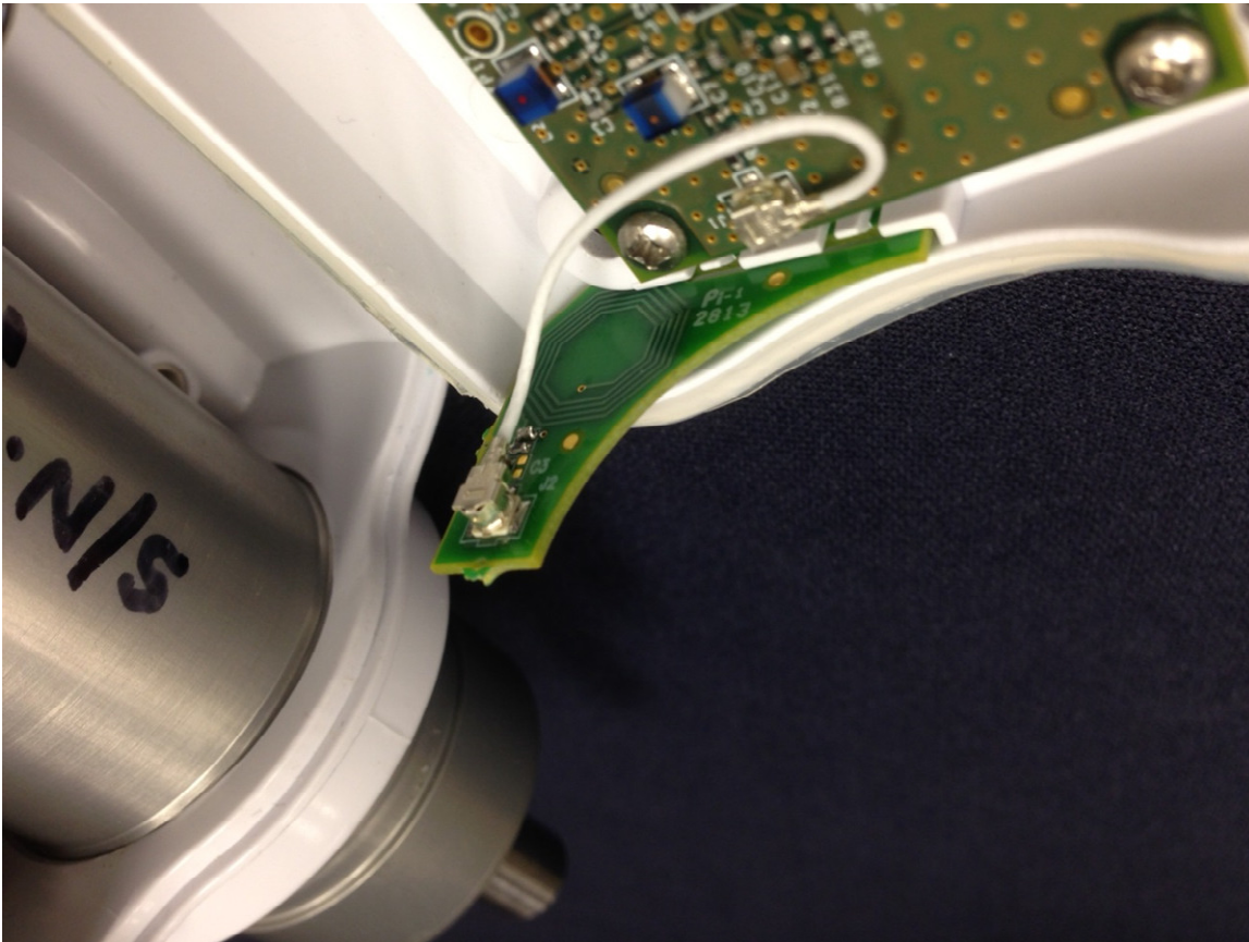
Figure 3: RF Board Mounted to TW Top Enclosure
