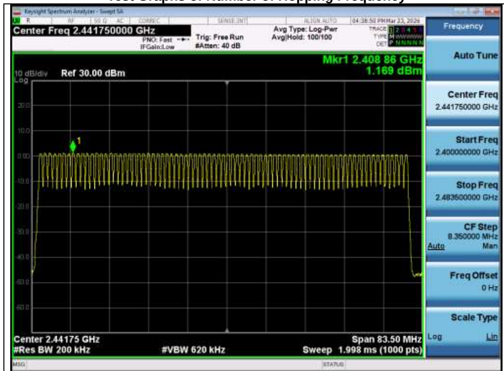
Test_Graph_BR_HOP_ANT1_NA_1Mbps_Number of Hopping
