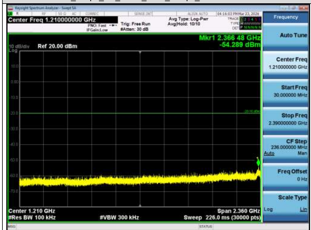
Test_Graph_BR_ANT1_2402_1Mbps_Lower Band Emissions
