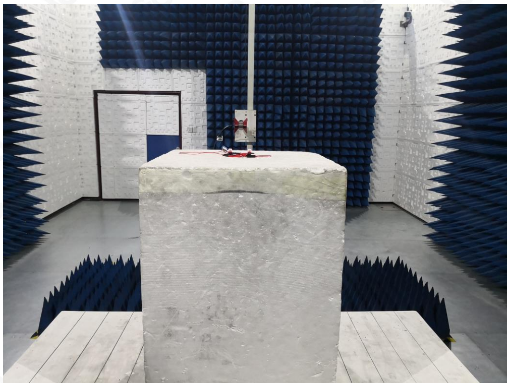
RADIATED EMISSION TEST SETUP ABOVE 1GHZ
