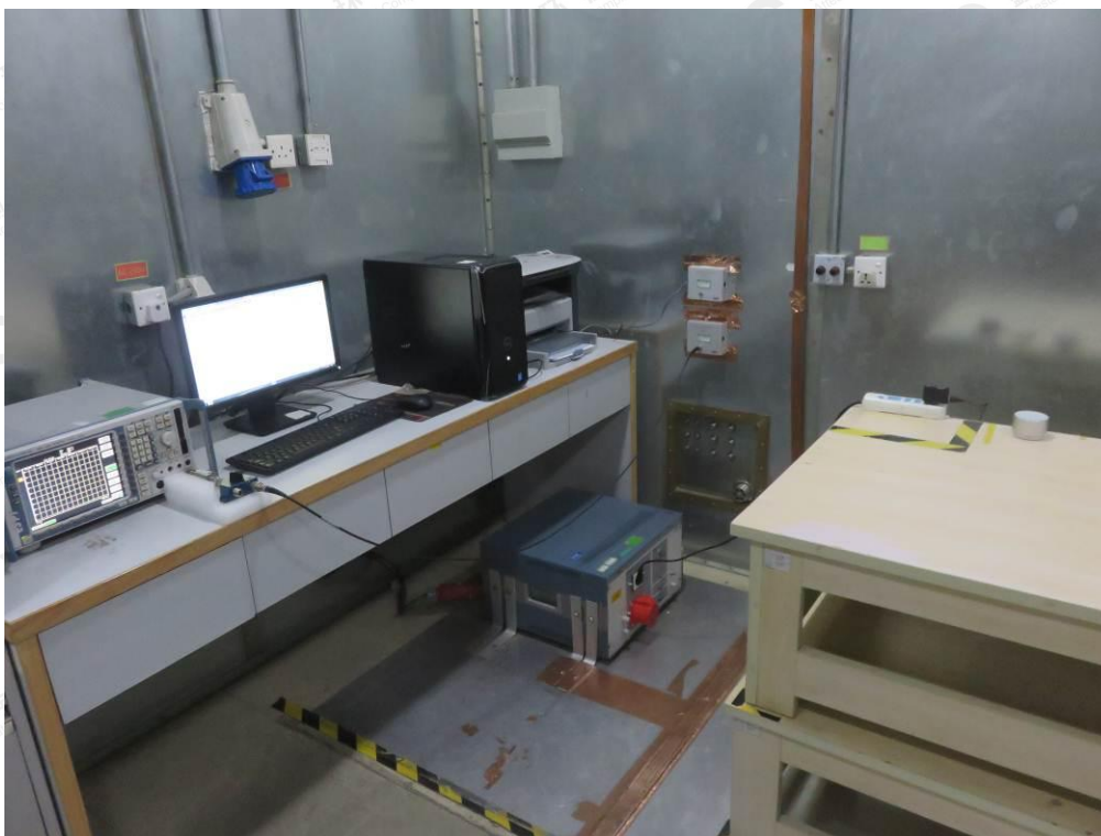
FCC RADIATED EMISSION TEST SETUP
