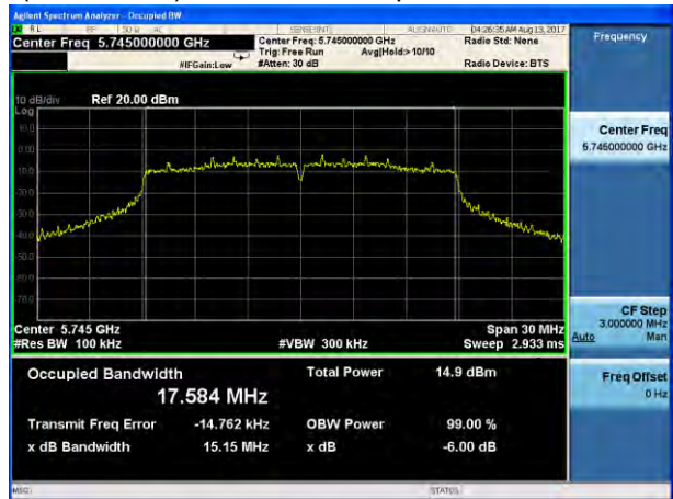
(802.11 n20) 6dB Bandwidth plot on channel 149
