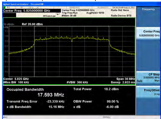
(802.11 n20) 6dB Bandwidth plot on channel 165
