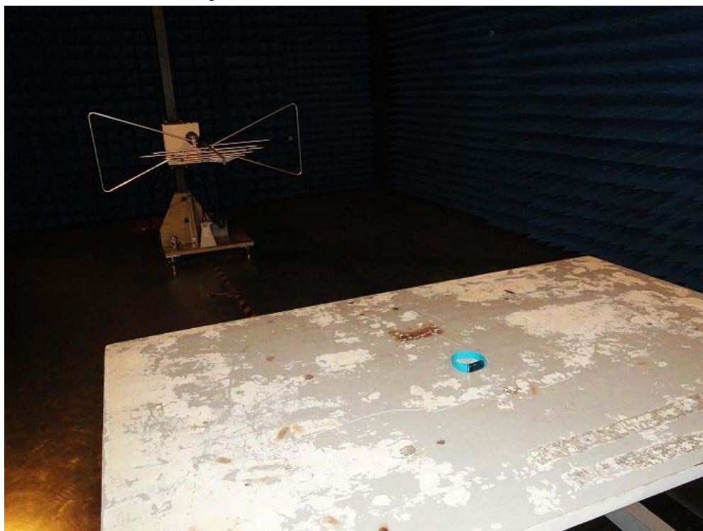
Radiated Emission Test Setup:
