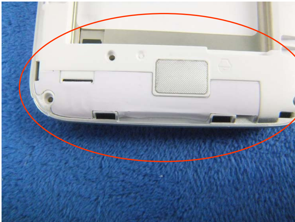
GSM/PCS/UMTS - Antenna View
