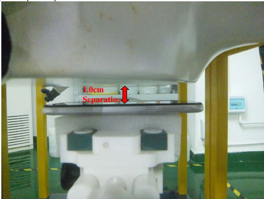
Body Setup Photo (LCD DOWN)
