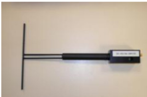
Figure 1 – Satimo COMOSAR Validation Dipole
