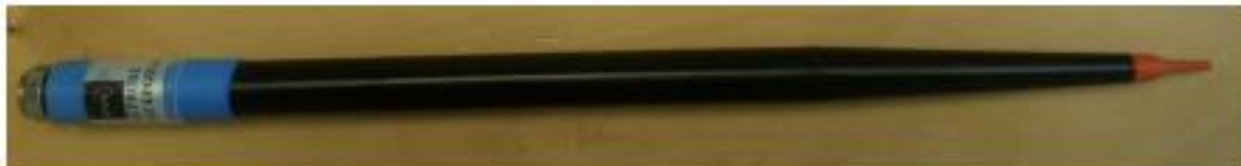
Figure 1 – MVG COMOSAR Dosimetric E field Dipole
