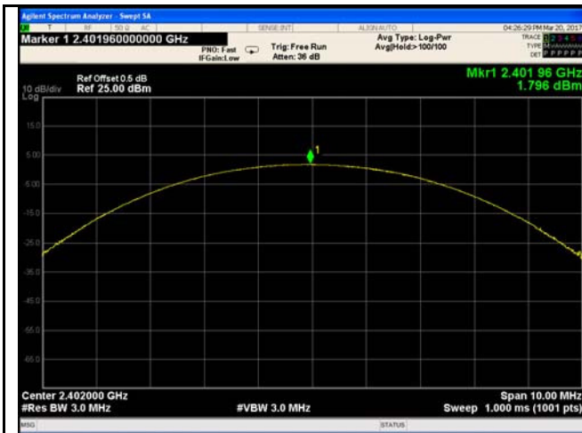
8DPSK Output power - Low CH 2402
